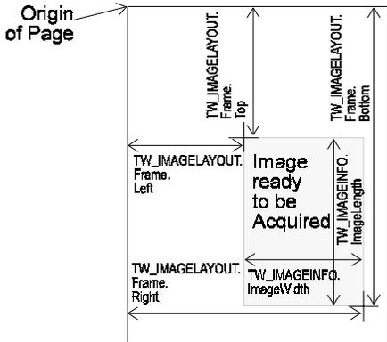
Figure 4-1. TW\_FRAME Structure
