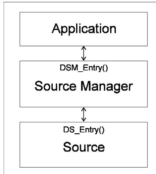
Figure 2-3. Entry Points for Communicating Between Elements
